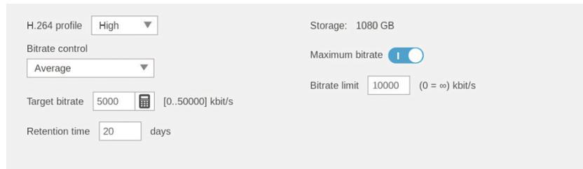
The screenshot shows a configuration interface for a camera. On the left, there is a section for 'H.264 profile' set to 'High', 'Bitrate control' set to 'Average', 'Target bitrate' set to '5000' kbit/s, and 'Retention time' set to '20' days. On the right, there is a 'Storage' section showing '1080 GB', a 'Maximum bitrate' toggle switch that is turned on, and a 'Bitrate limit' set to '10000' kbit/s.
