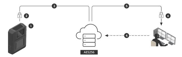
Secure live streaming with end-to-end encryption in AXIS Body Worn Live
