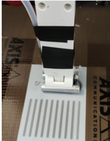
*Setup for the cleaning simulation. The samples were swiped with a cloth mounted on an automatic movable arm. The cloth was regularly resaturated with the chemical.*
