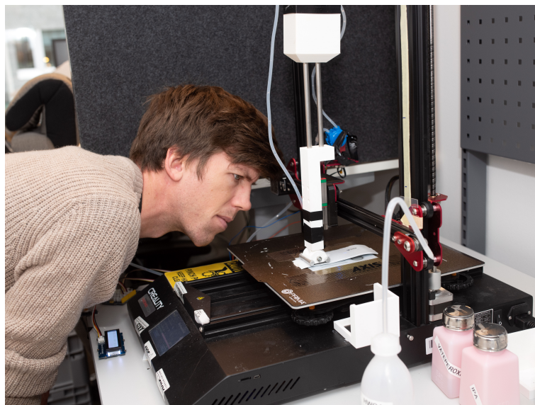
Figure 3.2 Set up for the cleaning simulation. The samples are swiped with a cloth mounted on an automatic movable arm.
