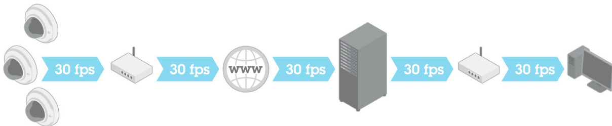
Figure 1. A surveillance system with a 30-fps controlled frame rate in every step. The frame rate of the camera can be preserved throughout the system only if the overall system performance is sufficient.
