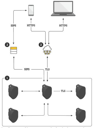
A network audio system with secure communication thanks to several open protocols.
