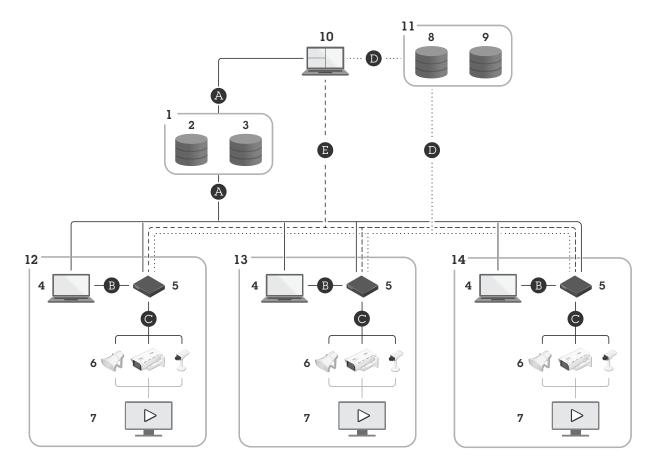
Typical setup for multisite operations with local and remote access using AXIS Device Manager Extend.
