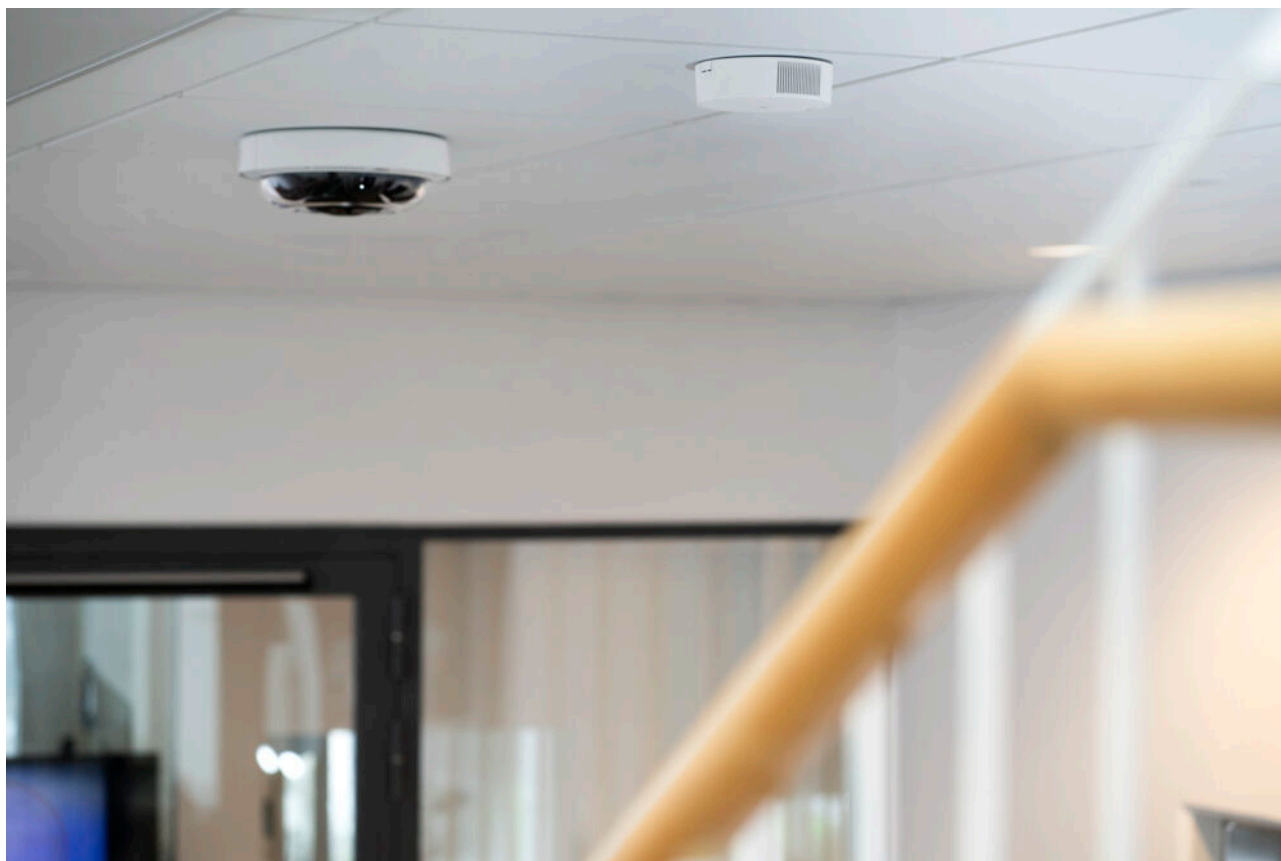
An air quality sensor and a camera that serves as host device.
