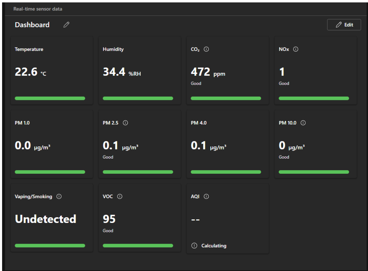
Dashboard showing live measurement data from an Axis air quality sensor.
