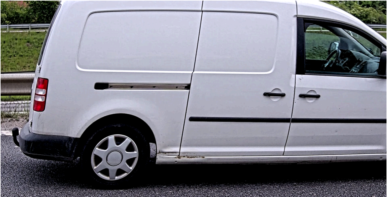
Figure 3.3 A car passing quickly through the image will look tilted because of rolling shutter distortion.
