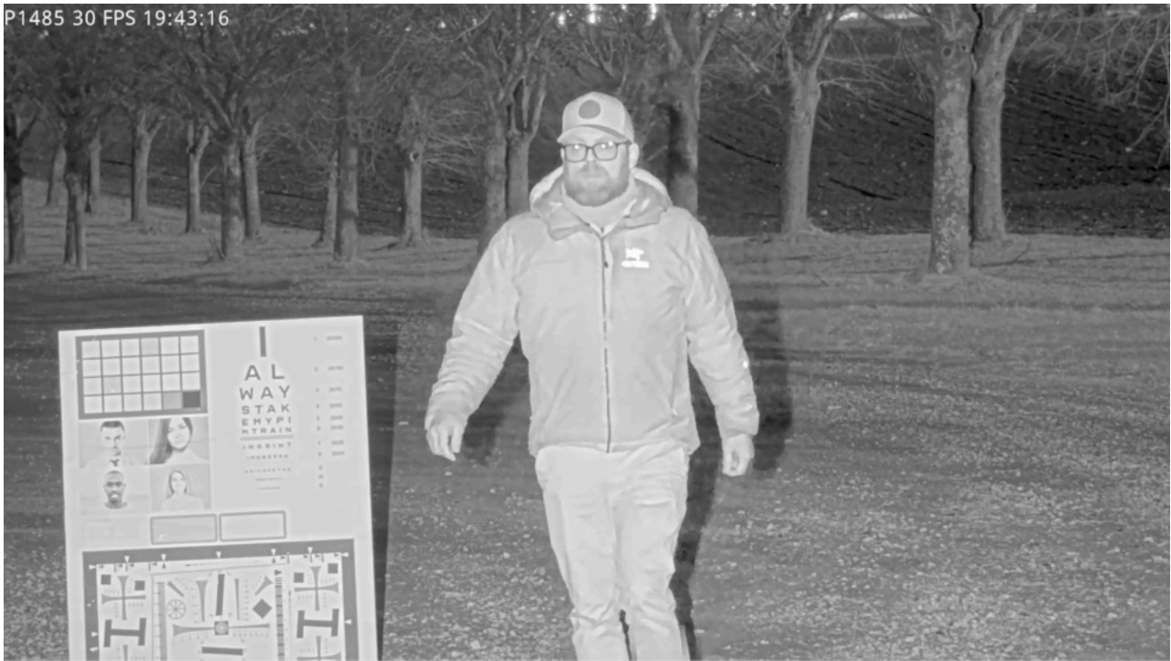
Figure 6.1 A rolling shutter camera with long exposure time ( 1/30 s) and a short IR-flash ( 1/1000 s). The IR-light is, in this case, visible in the full image since the flash occurs in the time interval where all rows of the sensor are simultaneously exposed to light.
