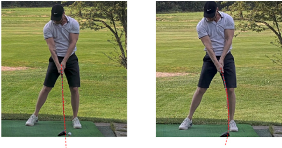
Figure 3.2 A golf swing captured at the same moment with a rolling shutter camera (left) and a global shutter camera (right). On the rolling shutter camera, the club looks bent due to rolling shutter distortion. Both cameras are set to very short exposure times of 1/10000 s to minimize motion blur.
