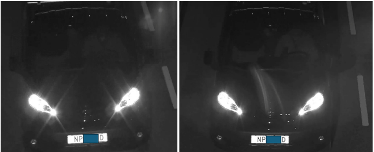
Figure 9.4 Car driving 70 km/h at night, illuminated by a 20 W continuous IR-source and captured by a rolling shutter camera and a global shutter camera with short exposure time (1/1000 s). The cameras have roughly the same light sensitivity and SNR.
