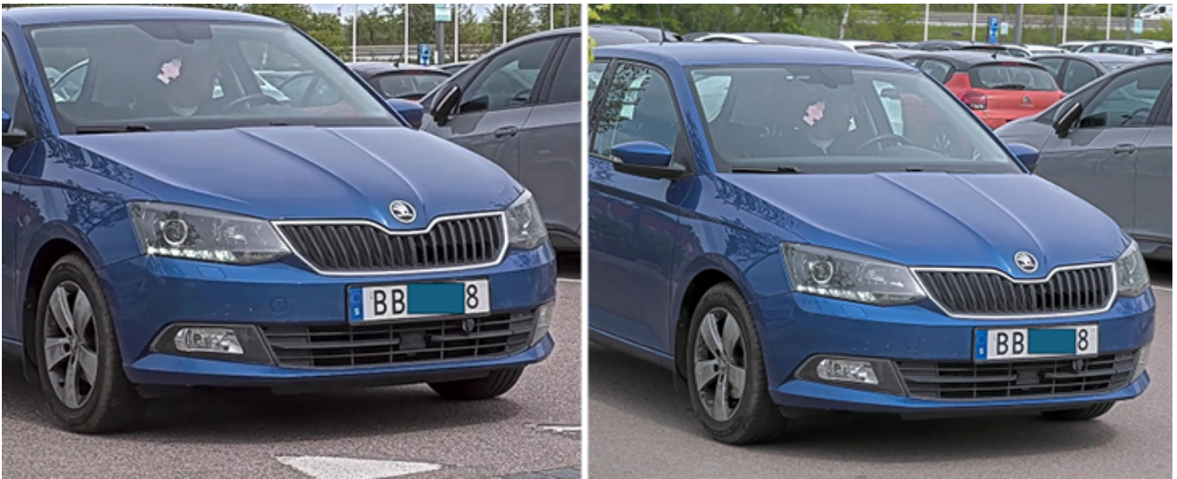
Figure 9.3 Car captured with a rolling shutter camera and a global shutter camera, with short exposure time (1/1000 s). Since motion through the image is very slow, there is no rolling shutter distortion. In this angle, rolling shutter is not visible.
