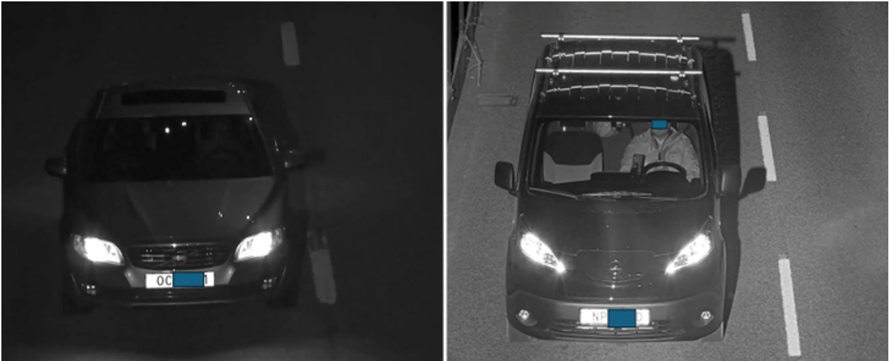
Figure 5.2 The first image shows a snapshot of a car taken with a rolling shutter sensor and a continuous IR-illuminator with 25 W power consumption. The second image is taken with a global shutter sensor and a strobing IR-illuminator with 20 W power consumption and 500 W peak power. Using a global shutter sensor together with strobing IR-light can drastically improve visibility.
