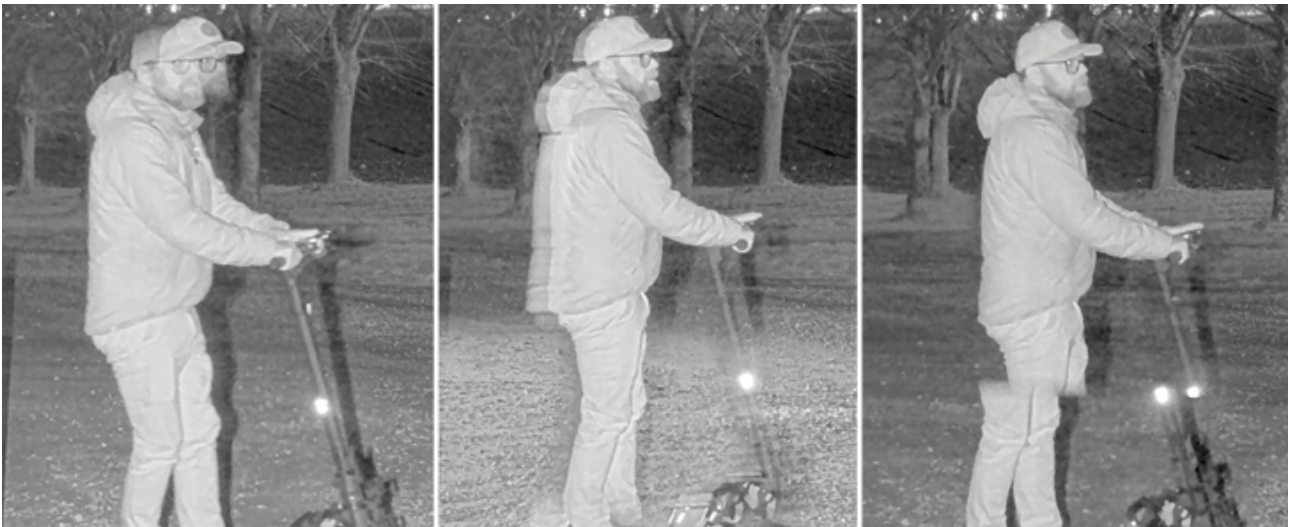
Figure 9.1 A rolling shutter camera with a long exposure time (1/30 s) next to a global shutter camera with strobing IR-light in WDR-mode. In WDR-mode, there will be two IR-flashes per frame, very close in time. The two pulses cause strange image artifacts on the rolling shutter camera, like double images, or cut images, of moving objects.
