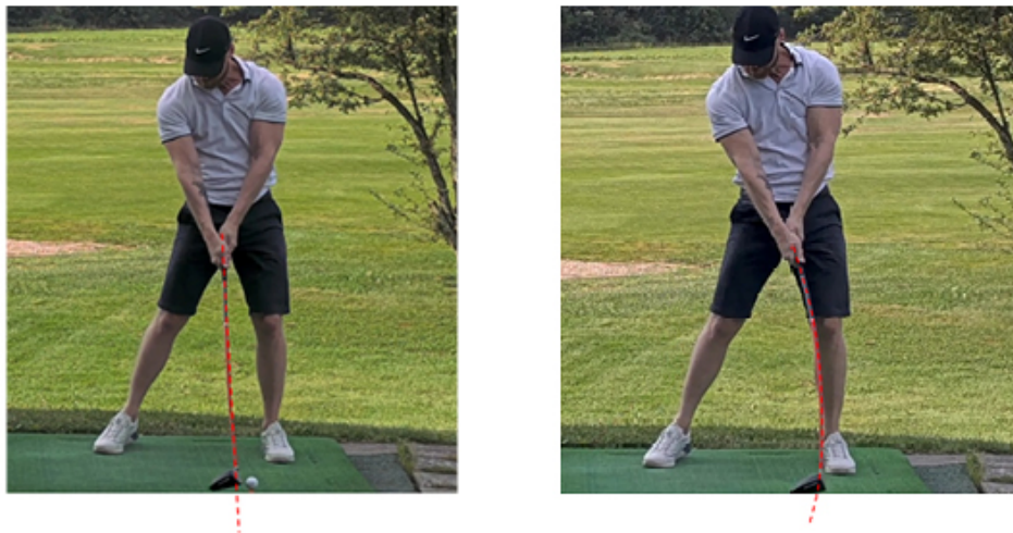
Figure 3.2 A golf swing captured at the same moment with a global shutter camera (left) and a rolling shutter camera (right). On the rolling shutter camera, the club looks bent due to rolling shutter distortion. Both cameras are set to very short exposure times of 1/10000 s to minimize motion blur.
