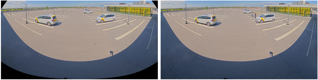
The areas in the corners of the image where there is no information from the image sensors can be preserved (displayed as black pixels) (left) or stretched (right) according to user preference.
