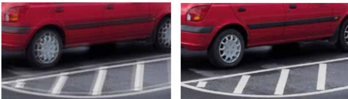
Figure 1. Simulated images. Left: a close-up without electronic image stabilization, showing both horizontal and vertical motion blur. Right: a snapshot from the vibrating camera with electronic image stabilization activated.
