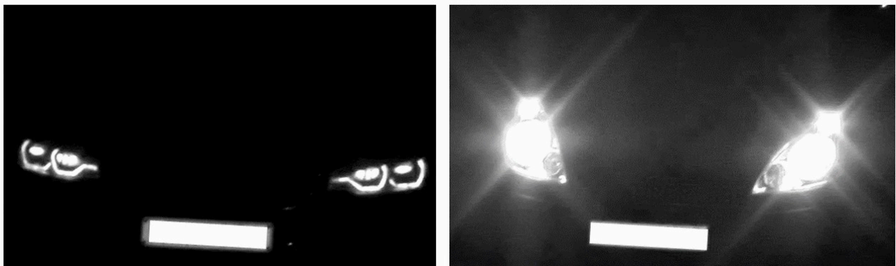
Two images taken almost simultaneously, with identical settings and alignment, using a camera equipped with IR-pass filter.
