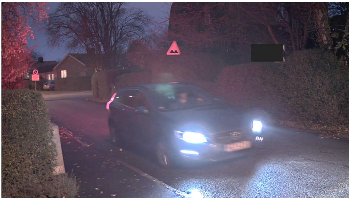
Figure 8. A long exposure time may cause visible motion blur. In this snapshot, the license plate might have been readable if a shorter exposure time had been used.
