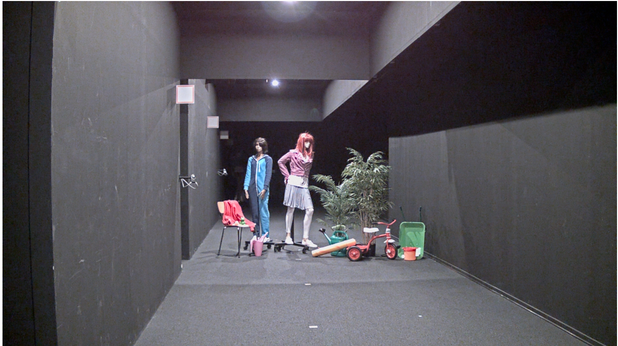
Figure 4. A studio scene with a light intensity between 1.5 lux (on the tricycle) and 5 lux (at mannequin waist height). The Lightfinder camera delivered clear colors and a deceptively bright image. The human eye could also discern color, but perceived the scene as being very dark.
