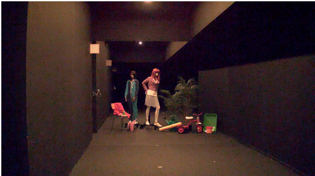
Figure 6. 0.1 lux – 0.3 lux measured on the objects. The Lightfinder camera provides a less sharp, but still very detailed, color image. The human eye could not discern the darker surfaces and perceived no details or colors.
