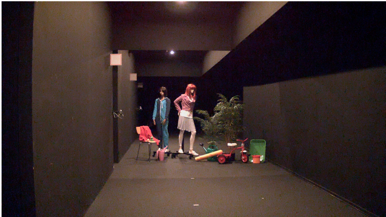
Figure 5. 0.2 lux – 0.7 lux measured on the objects. The Lightfinder camera provides bright colors. To the human eye, color vision was questionable, and mainly light surfaces could be discerned, with very little detail.
