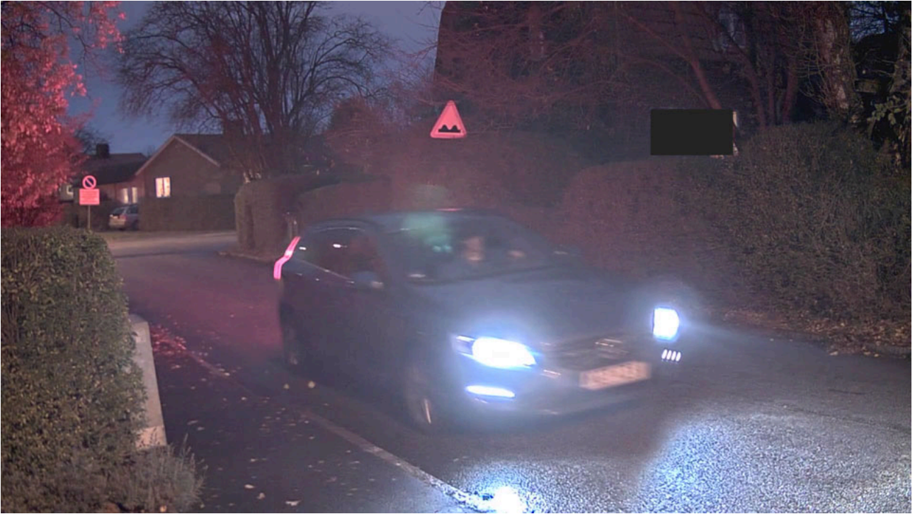
A long exposure time can cause visible motion blur. In this snapshot, the license plate might have been readable with a shorter exposure time.
