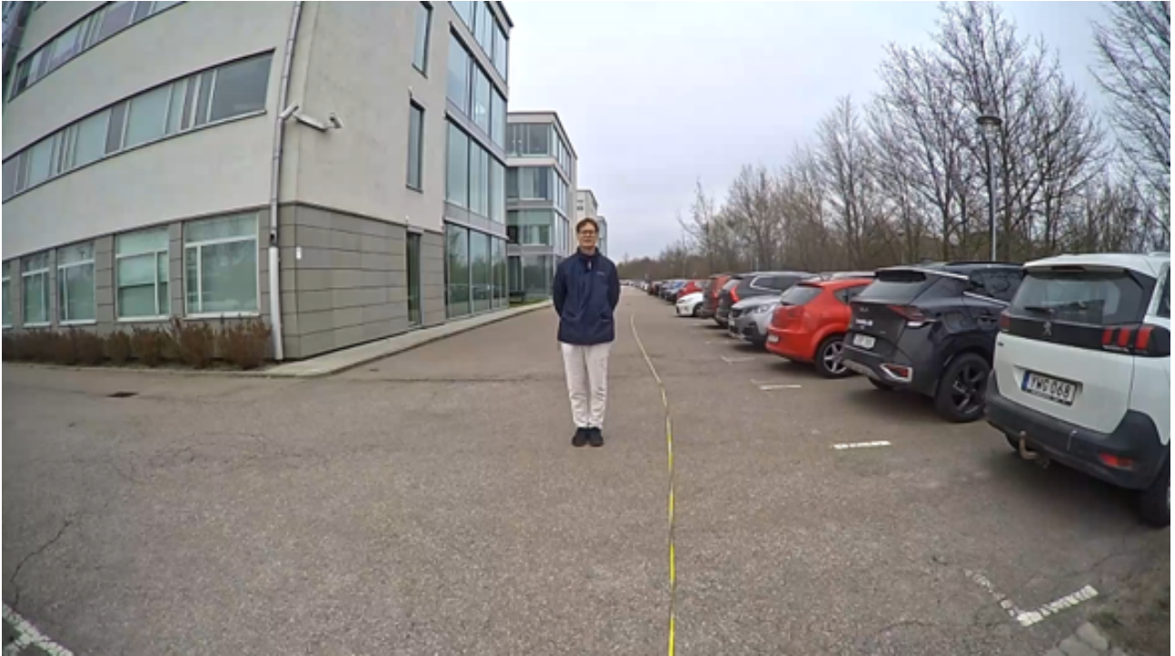
Figure 3.2 In the recording location, the maximum recording distance is 4 m away from an Axis body worn camera.
