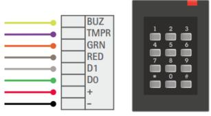
A Wiegand reader and its wiring, including extra cables for buzzer, tamper detection, and LEDs.
