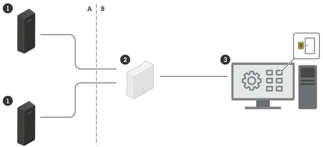
In physical access control, readers (1) are installed outside the door (non-secure area, A) and communicate with a door controller (2) installed on the inside (secure area, B).
