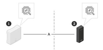
Achieving end-to-end security with secure keystore in access control. The master key and the individual secure channel base key (SCBK) are both stored in secure keystores, in devices on each side of the door.
