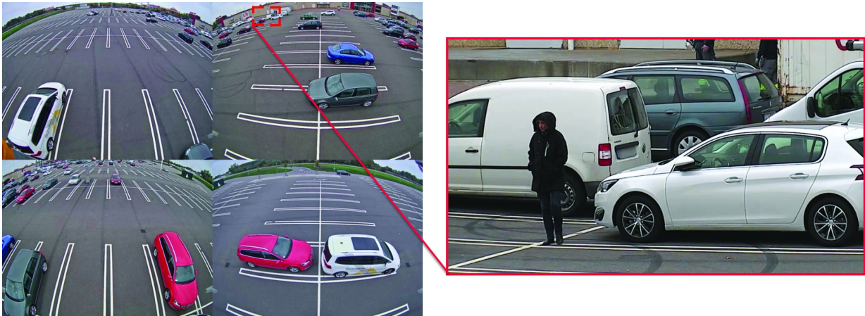
Parking-lot surveillance using a multidirectional camera with PTZ. Quad view 360° and PTZ zoomed-in view.
