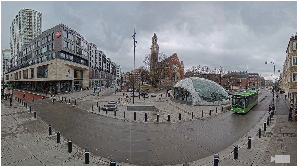
180° view (the street that looks curved is, in fact, straight) from a multisensor camera with four sensors.
