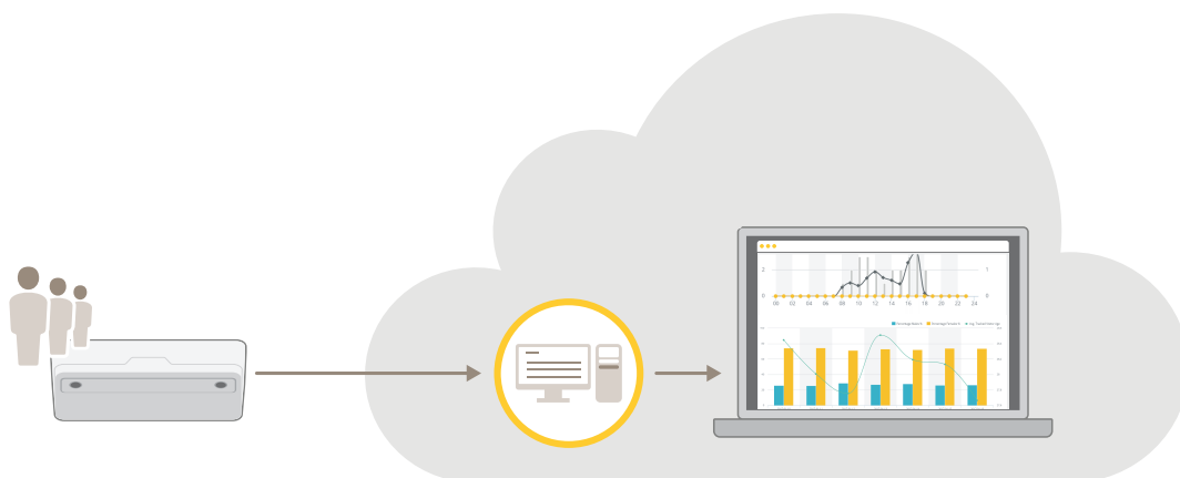
Figure 2. A people counting system requires a counting device and applications that manage and visualize the data.
