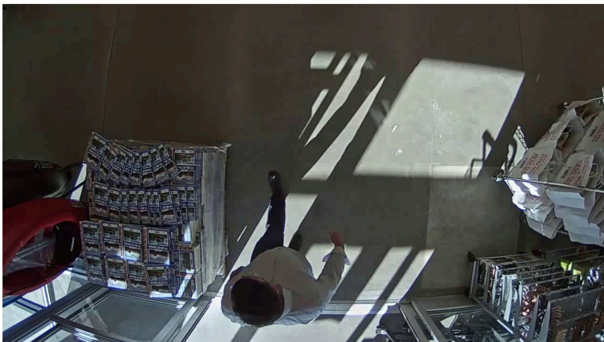
Figure 5. A scene with challenging light creating long shadows. A 3D people counter will immediately determine that the shadow has no depth, and discard it.
