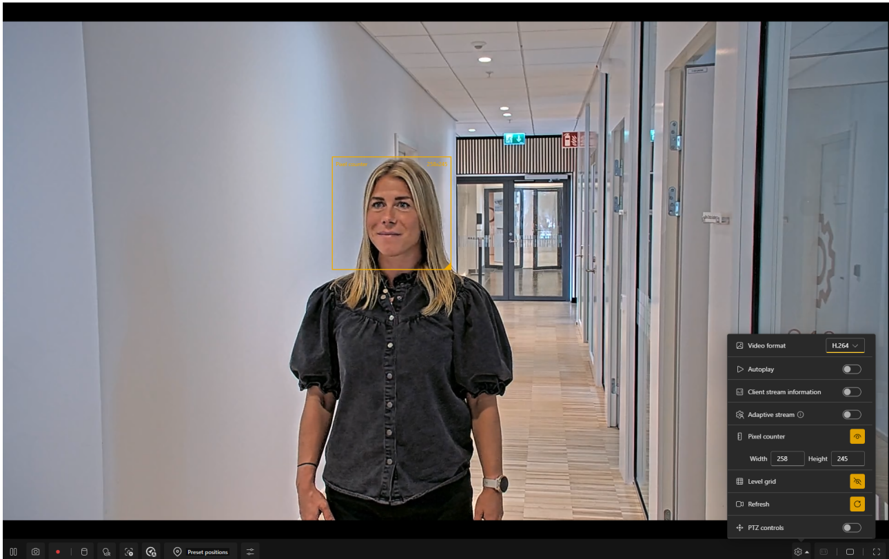
Figure 4.2 A camera view with the pixel counter visible. The tool shows that we have 96 pixels across the frame, which means that identification is possible (requiring at least 40 pixels across the face).
