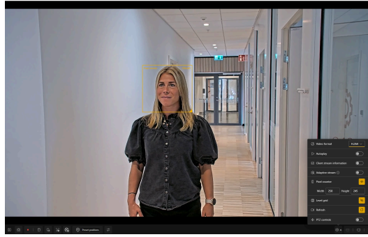
Figure 4.2 A camera view with the pixel counter visible. The tool shows that we have 96 pixels across the frame, which means that characterization is possible (requiring at least 40 pixels across the face).
