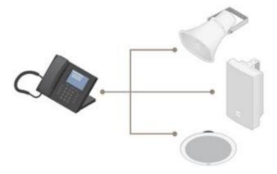
Most office telephones today are SIP-compatible. Any standard SIP telephone can be used to call the SIP address of an Axis IP audio device.
