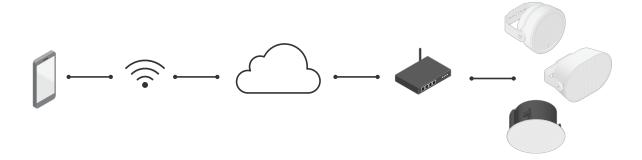
Paging via cloud is available with AXIS Audio Manager mobile app. This enables you to access your PA system from anywhere without requiring a paging station or handset. You can make general announcements and set volume and audio source from your mobile device.
