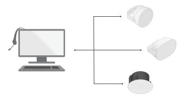
With a VMS (video management system) from Axis or an Axis software partner, you can use a USB headset connected to the VMS client as input device. Using the headset and a web button in the VMS client, you can make announcements to Axis speakers and trigger audio clips. This functionality is supported in AXIS Camera Station and many VMS solutions from Axis software partners.
