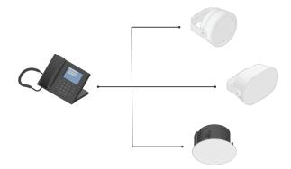
All office VoIP (Voice over IP) telephones today are SIP-compatible. Any standard SIP telephone can be used to call the SIP address of an Axis IP audio device.
