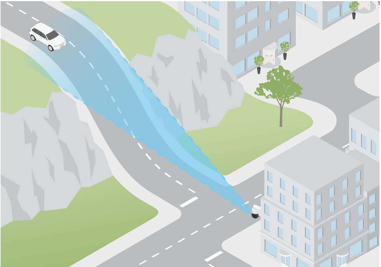
Figure 4.1 A PTZ camera with sharpdome is ideal in uneven terrain and open areas.
