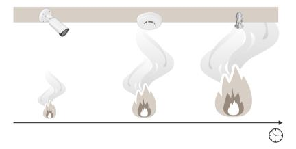
Fire detection based on video reacts faster than traditional smoke detectors.
