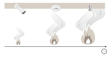
Fire detection based on video reacts faster than traditional smoke detectors.
