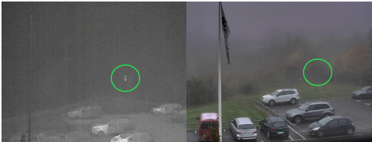
Images taken with a thermal camera (left) and a visual camera (right) on a foggy day. An individual (circled for reference) can be distinguished with the thermal camera but not with the visual camera.
