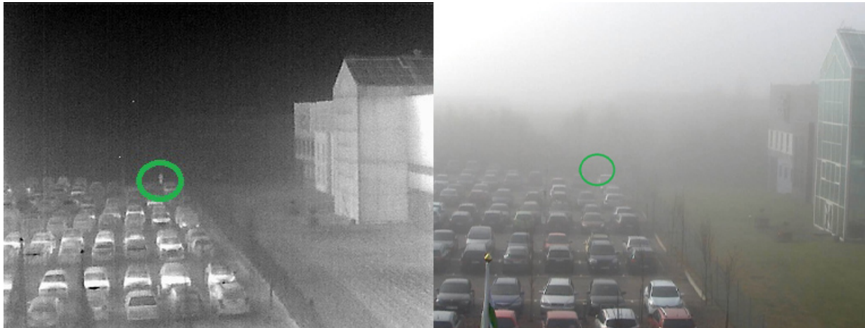
Image from a thermal camera (left) and a visual camera (right) on a misty day. A person (circled) can be distinguished with the thermal camera but not with the visual camera.
