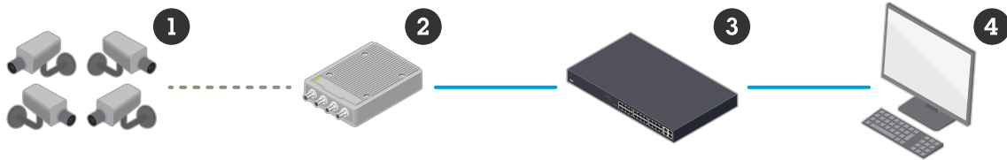
Figure 8. A network video system where video is continuously transported over an IP network. It uses a video encoder (2) as the cornerstone, along with a network switch (3) and a computer with a VMS (4), to migrate the analog security system into an open IP-based video solution.
