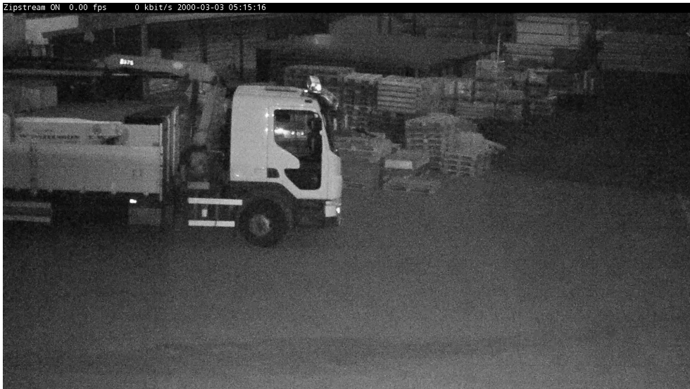
Above: night-mode scene with very infrequent motion. Total bitrate reduction: 99.7%. Zipstream strength: extreme. Dynamic GOP: on. Dynamic FPS: on.
